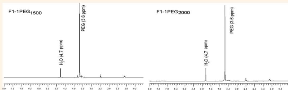
Figure 4. <sup>1</sup>H-NMR spectra of peptides of peptides F1-1PEG<sub>1500</sub> Y F1-1PEG<sub>2000</sub>. Signal to 3,6 ppm corresponds to protons of metilene groups of PEG.
