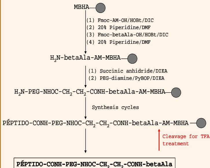
Figure 1. Methodology designed for obtaining the PEG-PS support for synthesis of C-terminal pegylated peptides.
